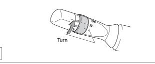
Front fog lights turn on only when the headlights are on low beam.
